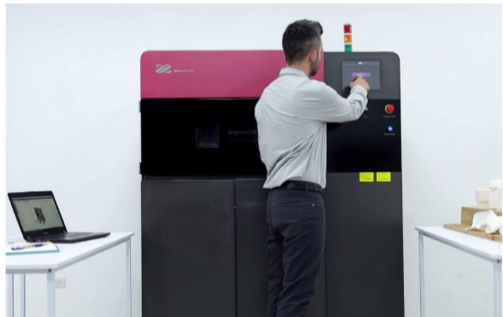
Figure 14. Desktop (left) and industrial (right) SLS 3D printing machine. Source: https://www.youtube.com/watch?v=oiEL4BGXQss Source: https://i.ytimg.com/vi/Y7Nj5NmTdEo/maxresdefault.jpg
