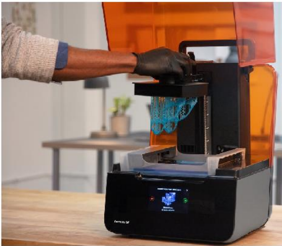
Figura 10. Impresora SLA de sobremesa (izquierda) vs. impresora SLA industrial (derecha). Fuente: https://formlabs-media.formlabs.com/filer_public_thumbnails/filer_public/be/50/be501495-9972-4536-9d27-57c0375b16a7/03062019_daguerre_1_565.jpg__1354x0_q85_subsampling-2.jpg Fuente: https://www.materialise.com/sites/default/files/styles/case_teaser/public/image-uploads/pages/Manufacturing/Technologies/3d-printing-technology_stereolithography.jpg?itok=DMgnH71i
