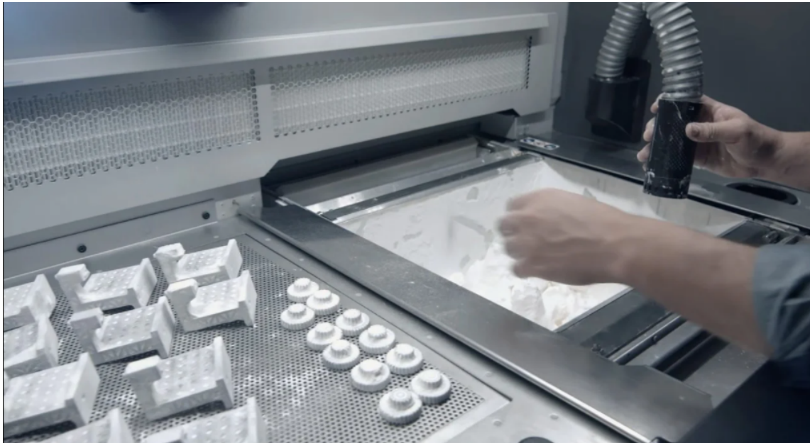
Figura 13. Estrazione e pulizia dei pezzi di una stampante 3D SLS. Fonte: https://i.all3dp.com/cdn-cgi/image/fit=cover,w=1284,h=722,gravity=0.5x0.5,format=auto/wp-content/uploads/2018/11/05175257/cleaning-the-powder-off-a-batch-of-items-printed-with-mjf-hp-youtube-181105.jpg
