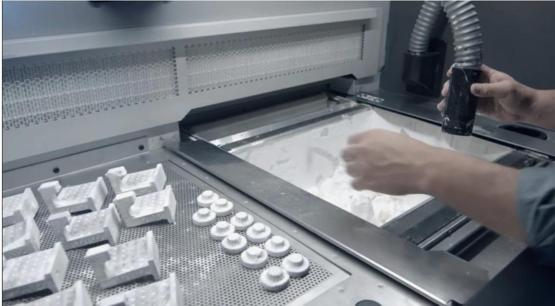
Figure 13. Extracting and cleaning pieces from a SLS 3D printer machine. Source: https://i.all3dp.com/cdn-cgi/image/fit=cover,w=1284,h=722,gravity=0.5x0.5,format=auto/wp-content/uploads/2018/11/05175257/cleaning-the-powder-off-a-batch-of-items-printed-with-mjf-hp-youtube-181105.jpg
