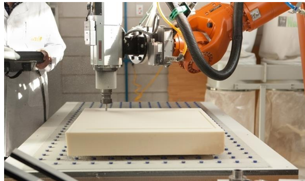
Figure 5. Subtractive manufacturing example. Source: CETEM.
