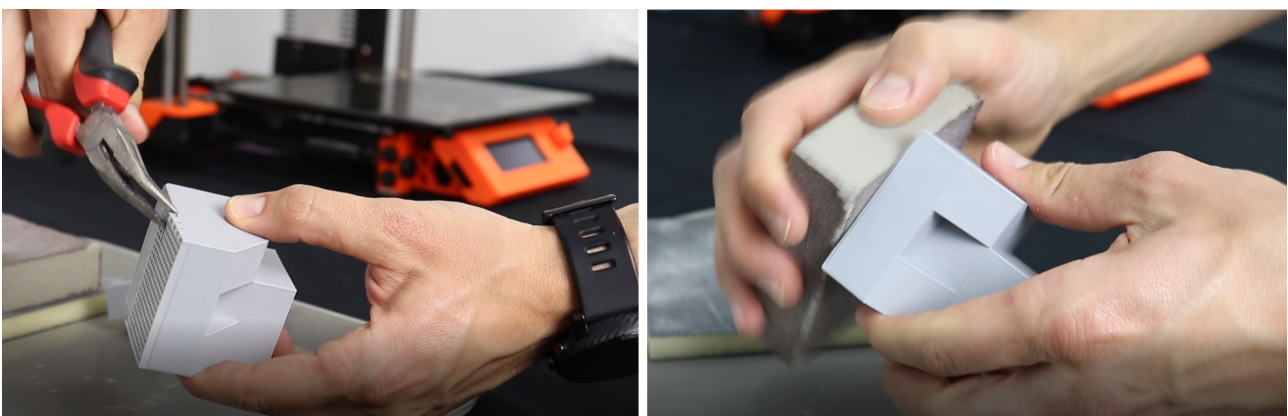
Figure 25. Removing supports structures from a FDM piece with pliers and sanding the surface. Source: CETEM.
